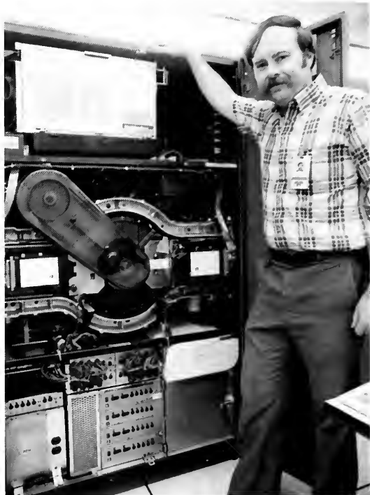
HEART OF Electronic Mail System is IBM 3081 mainframe which can hold 1.2 billion characters of information. Senior system programmer with Management Systems, Dan Dotson notes some 80 employees in 12 TRA departments are currently using EMS.
